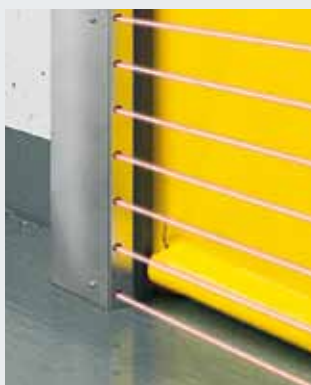
350-mm-high light grille concealed in the door guide
