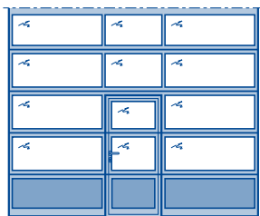
Sectional door ALR 67 Thermo with wicket door with trip-free threshold
